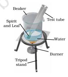
Figure 4.1 Set-up for extraction of chlorophyll
