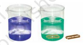
Figure 18.1 Change in colour of the copper sulphate solution due to reaction with iron (shaving blade)
