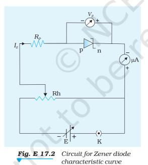
$V_z$  is termed as internal field emission which gives rise to a high reverse current or breakdown voltage. This breakdown is termed as *Zener breakdown* and the voltage at which it occurs is called *Zener voltage*. The reverse current at Zener voltage is called *Zener current*.
