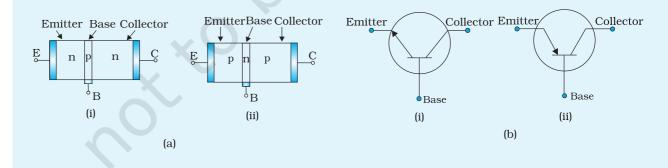
**Fig. E 18.1** (a) Schematic representations of n-p-n and p-n-p transistors along with their (b) circuit symbols
