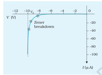
Fig. E 17.1 Zener diode characteristics curve
