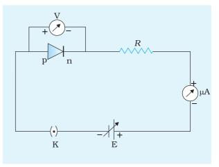
bias characteristics. Connect p-side **Fig. E 16.2** *Reverse biasing for a p-n junction diode*
