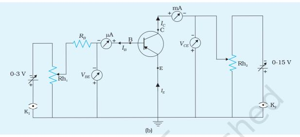
**Fig. E 18.3** Circuit diagram for studying the characteristics of (a) n-p-n transistor (b) p-n-p transistor, in CE configuration
